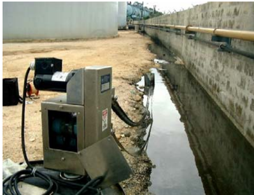
At a site in the Caribbean, the NTST series NET™ system was adapted to recover a surface spill of petroleum products within an above ground storage tank farm.
